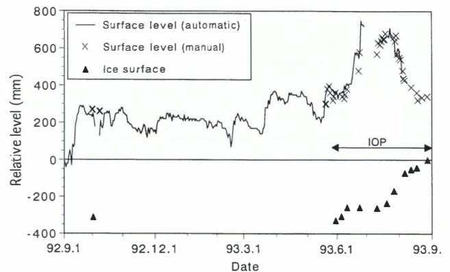
Fig. 4. The variation of surface level and ice-surface relative to the mass-balance stake at 5600 m a.s.l. on Xiao Dongkemadi Glacier from September 1992 through August 1993.
