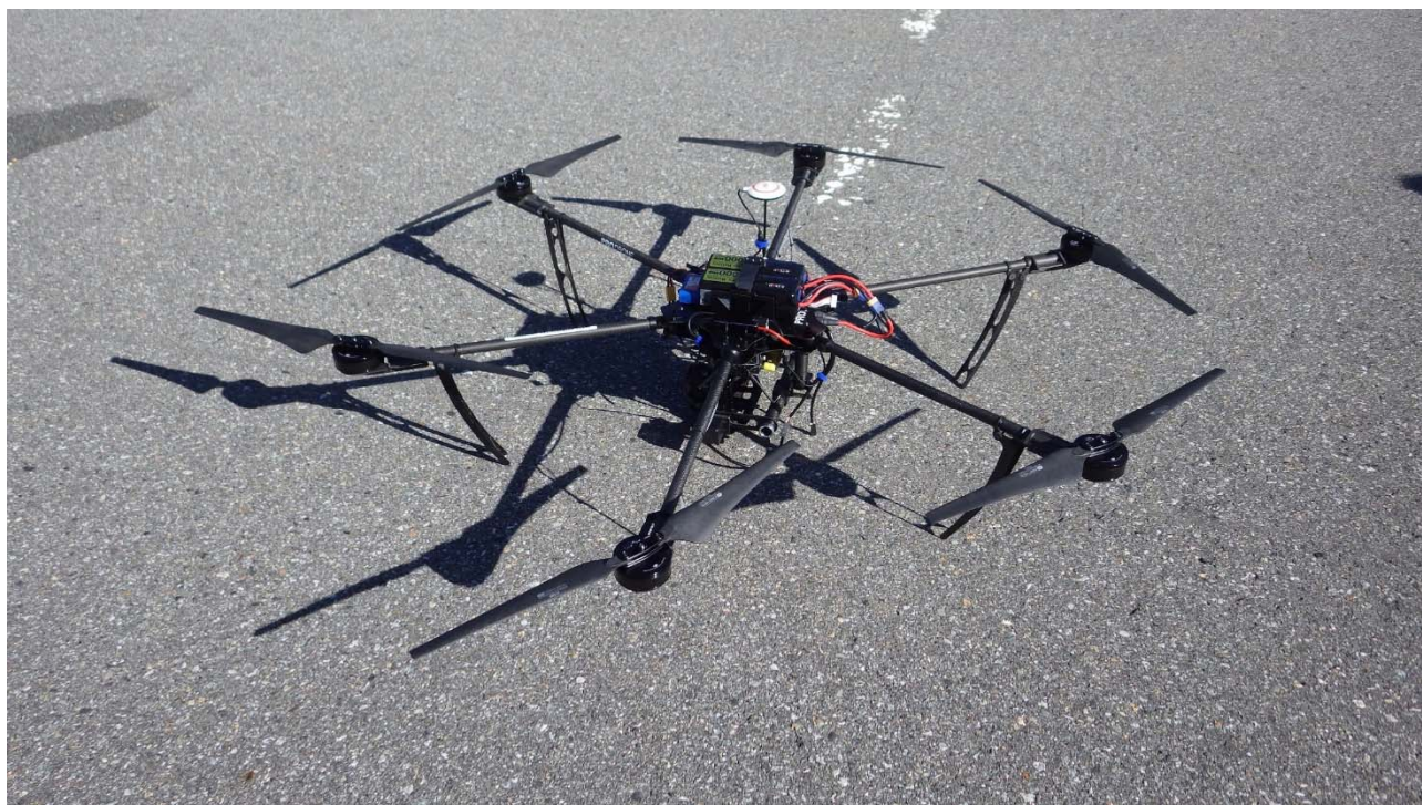
Fig. S1. Image of the hexacopter (PD6-NPL) used in this study. The greatest width is \sim 1.2 m.
